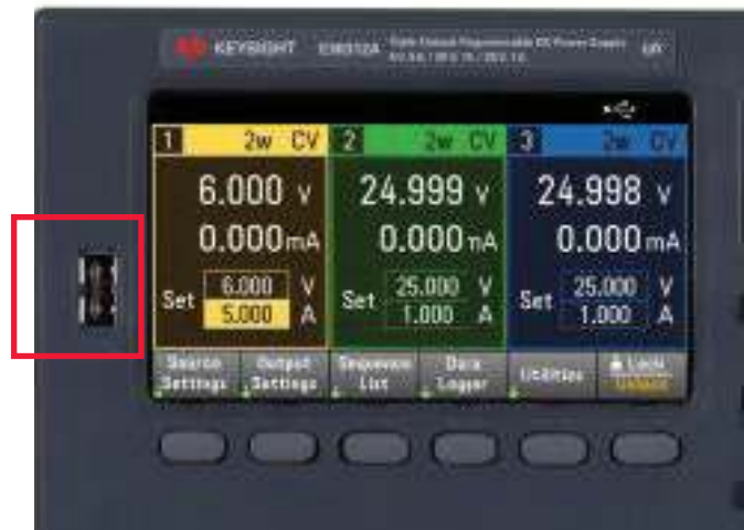
Figure 7: USB port on the front panel
