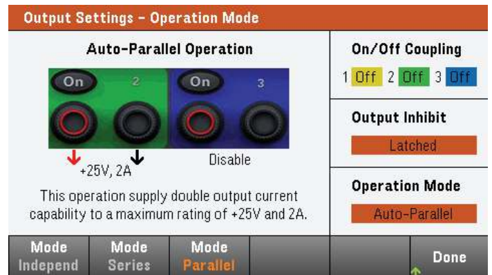
Figure 4. Auto-parallel operation to double the output current
