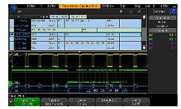
Figure 19. Multi-bus time aligned decode.
